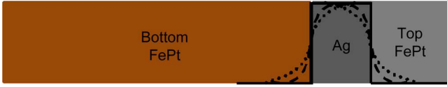
Fig. 1. Schematic illustration of the dependence of Ag/FePt intermixing on intermixing factor a . Absence of intermixing when a = 0 (solid line). The extent of intermixing increases with increasing value of a , when a > 0 (dashed line to dotted line).
